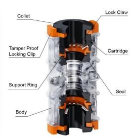
**Application** Straight connectors for DB (Direct Buried) microducts. Suitable for direct buried
