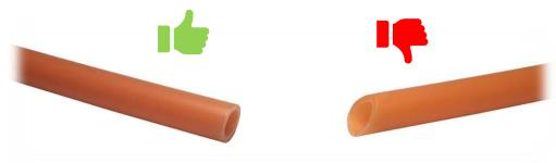
Make sure that the microduct is clean and does not contain any scratches, cracks, cuts or deformities on its surface.
